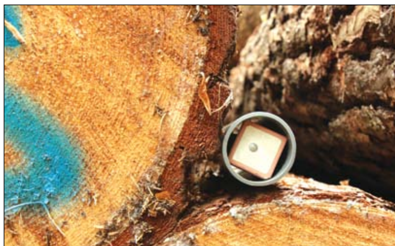
Picture showing the tracking module, which is normally inserted into a hole drilled in the end of a log.
