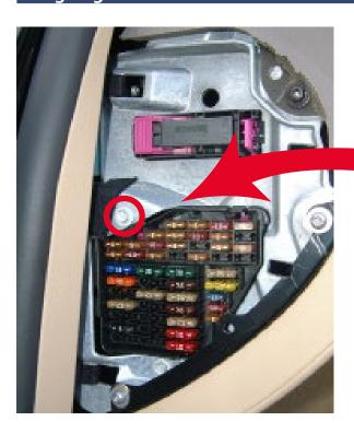
ENAiKOON locate-19 is easy to connect directly to the power supply, simply connect your lead to the main earth depole screw and plug the positive lead/fuse plug into a fitting vacant slot.
