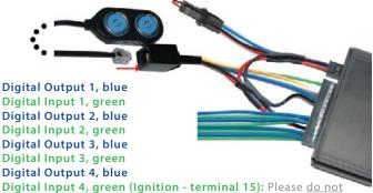
Digital Input 4, green (Ignition - terminal 15): Please do not connect it to the car radio or to the terminal 15r or terminal 30z or to the cable with tension of the ignition switch 1, connect it directly to the terminal 15 and to the cable with tension of the ignition switch 2
