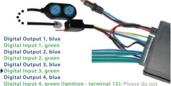
Digital Input 4, green (Ignition - terminal 15): Please do not connect it to the car radio or to the terminal 15r or terminal 30z or to the cable with tension of the ignition switch 1, connect it directly to the terminal 15 and to the cable with tension of the ignition switch 2
