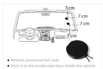
Please ensure that there is no material between the ENAiKOON locate-06 antenna and the sky that may interfere with the radio transmission, such as metal, water, metal oxide windscreens, or plastic with a metal varnish.
