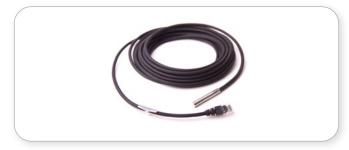
The temp-sensor attaches to the ENAiKOON locate-06 and can measure temperatures from -55°C to +125 °C (-67 °F to 257 °F) to an accuracy of 0.5°C (0.9 °F). Up to 16 temperature sensors can be simultaneously attached to an ENAiKOON locate-06 remote monitoring device without affecting its output.
