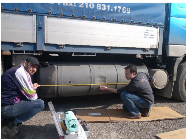
Picture 9: finding the geometric centre of the tank
