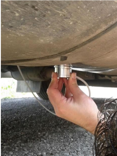
Picture 14: press the sensor to make the glue layer thin and bring the sensor closer to the tank bottom
