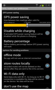
Using a slide bar the time can be set between GPS readings by GPS receiver. The greater the number, the more power is saved, but the routes recorded are only as detailed as the frequeny of the GPS readings. This power saving mode can be set depending on the wether the device is charging and the battery level.
